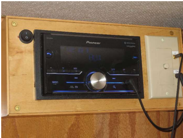
Rear stereos can be switched between Television and house audio from cab stereo
