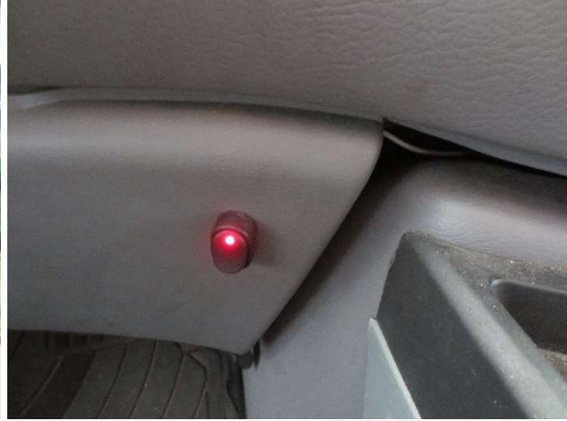
Ignition bypass for radio so no key is needed runs on House batteries
